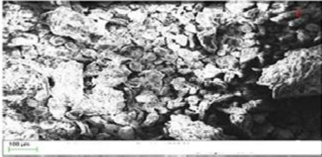
Figure 4. Morphological images of carbon powder
